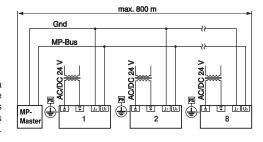
The actuators are supplied locally with AC 24 V via a separate transformer. The cable lengths of the MP cables indicated in the table apply regardless of the performance data of the connected actuators (see general notes).
