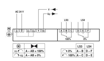
Electrical installation for 3-lead connection
