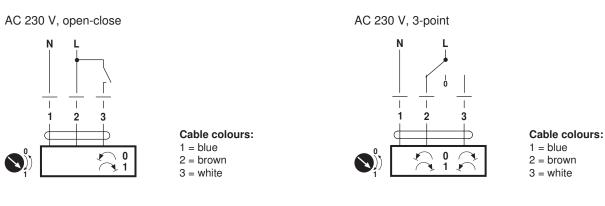
Damper actuator, IP66 + IP67, Open-close, 3-point, AC 230 V, 20 Nm
