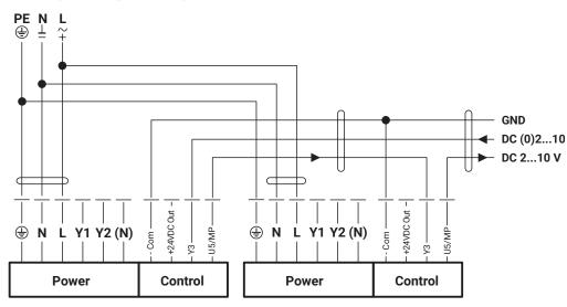
Power supply must not be connected to the signal terminals!
