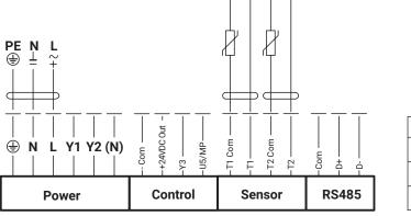
Connection of active sensors (BACnet MS/TP / Modbus RTU)
