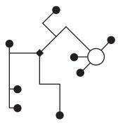
There are no restrictions for the network topology (star, ring, tree or mixed forms are permitted). Supply and communication in one and the same 3-wire cable • no shielding or twisting necessary
