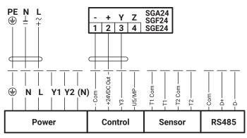
Note Maximum output power «+ 24VDC out» 1.2 W @ 50 mA! A separate safety transformer must be used for higher performance!
