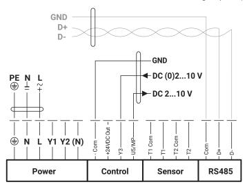
Connection of passive sensors (BACnet MS/TP / Modbus RTU)
