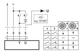
Globe valve actuator fail-safe, modulating, communicative, AC/DC 24 V, 1000 N, Running time motor 35 s
