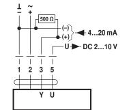
Control with 4...20 mA via external resistor
