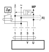
Connection of external switching contact
