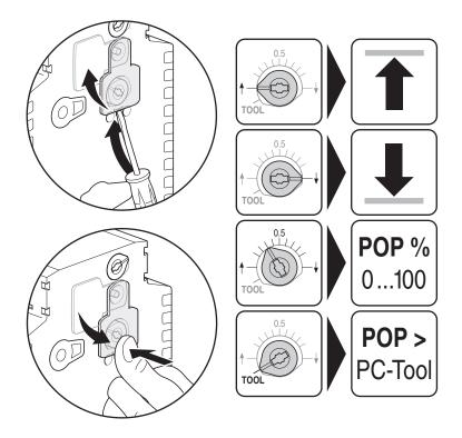
Globe valve actuator fail-safe, modulating, communicative, AC/DC 24 V, 1000 N, Running time motor 35 s
