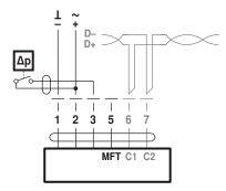
Requirements for switching contact: The switching contact must be able to accurately switch a current of 16 mA @ 24 V.
