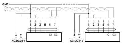
Connection with passive sensor, e.g. Pt1000, Ni1000, NTC
