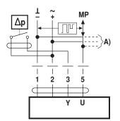
Connection of external switching contact
