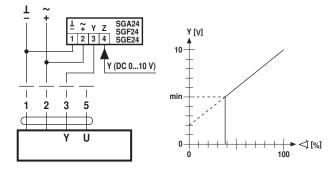
Control remotely 0...100% with positioner SG..
