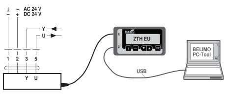
Globe valve actuator, modulating, communicative, AC/ DC 24 V, 500 N, Running time motor 35 s
