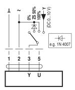
Control remotely 0...100% with Minimum limit with positioner SG.. positioner SG..
