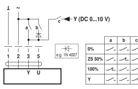
Override control with AC 24 V with rotary switch
