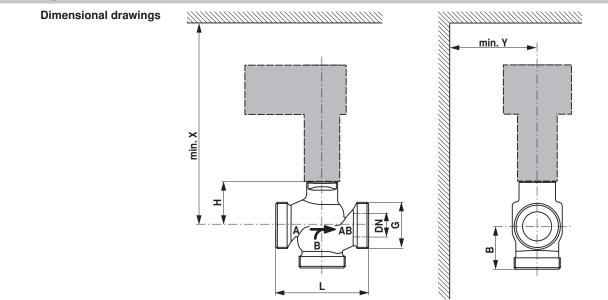
X/Y: Minimum distance with respect to the valve centre. The actuator dimensions can be found on the respective actuator data sheet.
