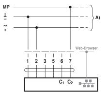
MP-Bus via 2-wire connection, local power supply
