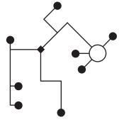
There are no restrictions for the network topology (star, ring, tree or mixed forms are permitted). Supply and communication in one and the same 3-wire cable • no shielding or twisting necessary
