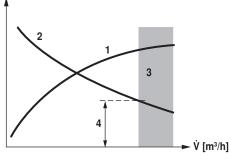
Power output of the heating or cooling registers 1 Diff. temperature between supply and return 2 Loss zone (heating or cooling register saturation) 3 Adjustable minimum differential temperature 4
