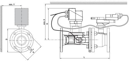
If Y <180 mm, the extension of the hand crank must be demounted as necessary.
