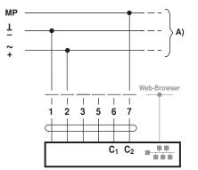
MP-Bus via 2-wire connection, local power supply
