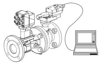
This can be inverted in cases of control with an analogue positioning signal. The inversion causes the reversal of the standard behaviour, i.e. at a positioning signal of 0%, regulation is to V'max or Q'max, and the valve is closed at a positioning signal of 100%.
