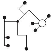
There are no restrictions for the network topology (star, ring, tree or mixed forms are permitted). Supply and communication in one and the same 3-wire cable • no shielding or twisting necessary
