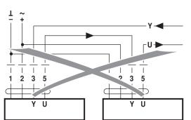
Control with 4...20 mA via external resistor
